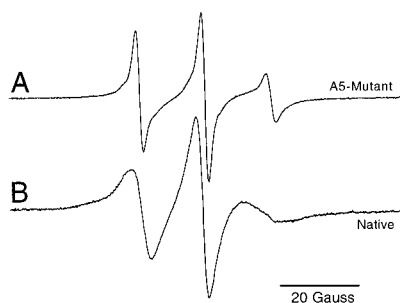
FIGURE 4: Comparison of the EPR spectra for MARCKS-derived peptides fully bound to 1000 Å lipid vesicles at a PC/PS ratio of 3:1: (A) The phenylalanine to alanine derivative, MARCKS-Ala, labeled at position 23 (N23C-R1), and (B) the native MARCKS-(151-175) also labeled at position 23 (data taken from ref 23). The peptides are at a concentration of approximately 100 μM and the lipid is at a concentration of 100 mM.
